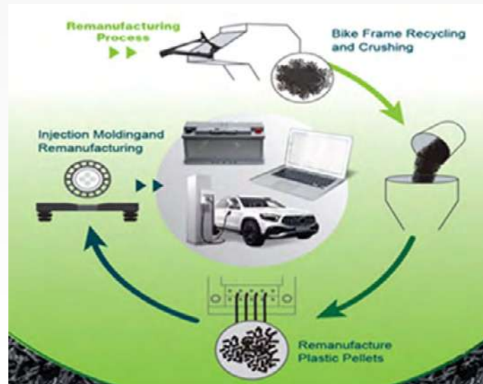
Caption | HYC thermoplastic carbon fiber product recycling and reuse process
