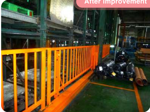
Caption | After improvement: replaced with rigid protective barrier
