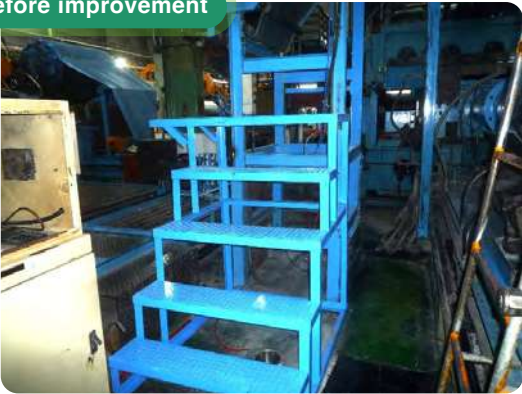
Caption | Before improvement: insufficient width of operational staircase
