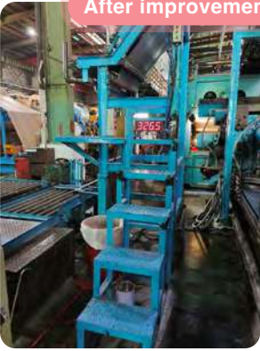
Caption | After improvement: rebuilt staircase to widen operational staircase width
