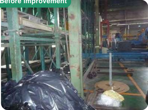
Caption | Before improvement: protective barrier used steel cables with inadequate strength
