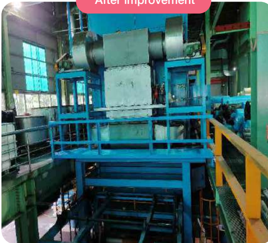
Caption : After improvement: replaced with protective barrier.
